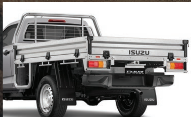
Heavy Duty Steel Tray - All Heavy Duty Tray features in sturdy steel with tie-down shackles built into the tray floor. Colour coding optional for cab chassis models.
